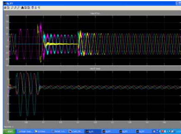
Fig.4- Fault occurrence in blue phase
